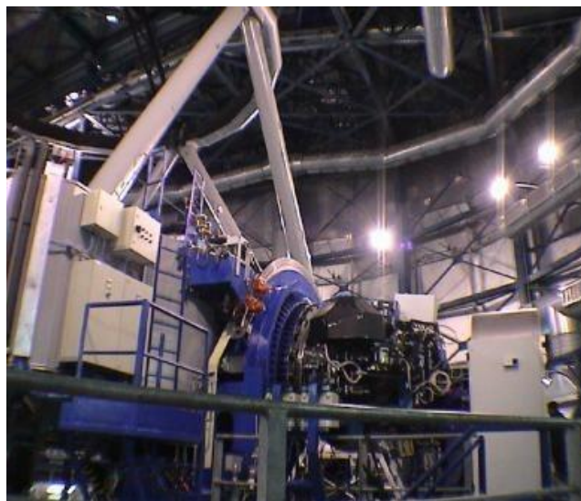
The VIMOS spectrograph mounted on the Nasmyth focus of the UT3 Melipal telescope of the VLT. Credits for the photo European Southern Observatory ESO / G. Sciarretta.
