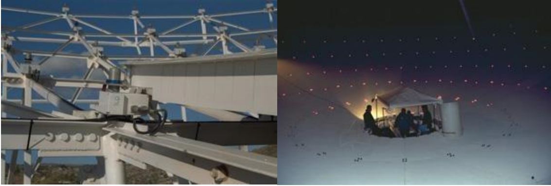
One of the panels of the Noto antenna (SR) supported by an actuator (left); measurements on the parabolic surface were carried out at night to minimize thermal effects on the mirror structure (right). Credits: INAF-IRA
